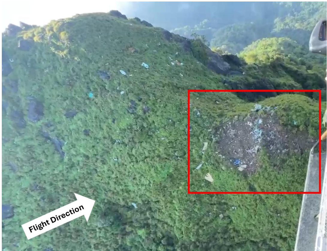
Figure 10: Initial impact mark (inside the red square) with illustration of the flight direction
